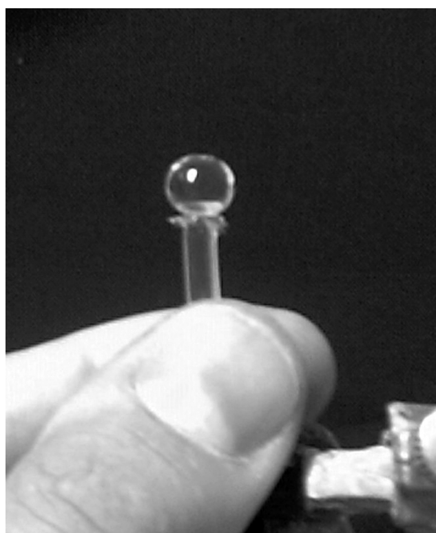
Figure 1 Customized balloon made of latex, fixed on top of a rigid catheter. The catheter was attached to a pump system to simulate the fetal cardiac phases.
